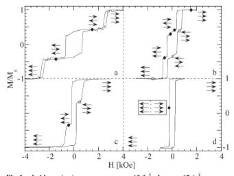
**Fig. 1a–d.** Magnetization curves, **a**  $t_{Cr} = 12.3$  Å, **b**  $t_{Cr} = 17.6$  Å, **c**  $t_{Cr} = 23$  Å, **d**  $t_{Cr} = 31$  Å. *Arrows* indicate the direction of the three Fe layer magnetizations as measured (•) or inferred (•) by symmetry at different fields by PNR. For (**a**), (**c**), and (**d**) the saturation configuration was measured at 5.4 kOe
