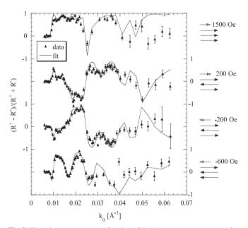
**Fig. 2.** The spin asymmetry as a function of incident neutron momentum for  $t_{Cr} = 17.6$  Å and the determined orientation of the Fe layer magnetizations. The difference in the spin asymmetry at +200 Oe and -200 Oe, is simply a difference in sign due to the switched sign of the applied field, which defines the "+" state of the neutron spin
