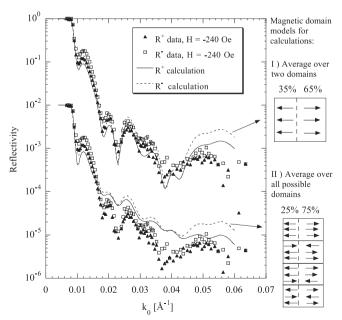
**Fig. 3.** The spin dependent reflectivities as a function of incident neutron momentum for  $t_{Cr} = 31$  Å measured with the field along the *easy axis*. The same data is compared to two calculations, each assuming a mixture of domains. The top model best corresponds to the data
