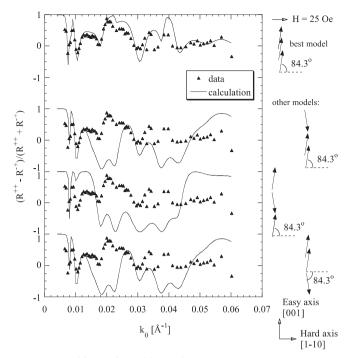
**Fig. 4.** The  $(R^{++} - R^{-+})/(R^{++} + R^{-+})$  as a function of incident neutron momentum for  $t_{Cr} = 31$  Å measured with the field along the *hard axis*. The same data is compared to four calculations. The top one best represents the data
